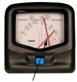
Correct SWR reading: the crossing pointer (SWR=1.7)
